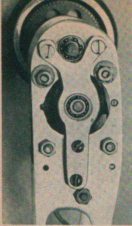
8) Right-hand motor bearing mount is removable so armature can be dismantled through \frac{3}{4} -inch hole in frame side piece.
