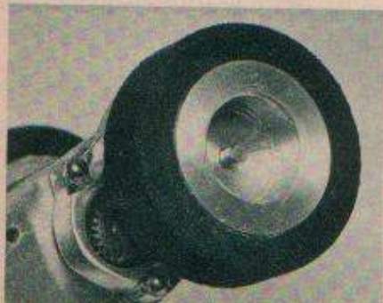
5) Mag rear wheels are Raceway experimentals with German record plane tires.
