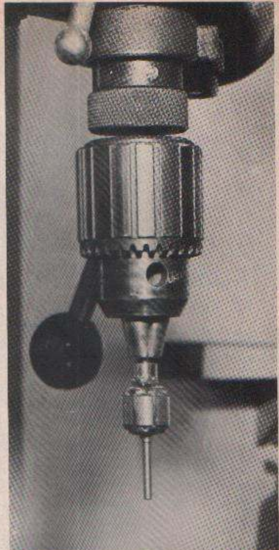
9) Place stock armature in drill press, set for slow speed, turn on and check armature shaft for straightness. If the shaft wobbles, correct this until it is straight and then switch armature ends in the drill press and check the other end. About one third of the shafts I've seen were bent and needed straightening.
