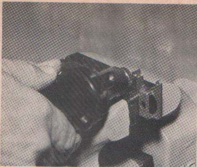
4) Using a Dremel power tool or files, remove area as indicated to lighten right hand endplate. Now cut back half of endplate off.
